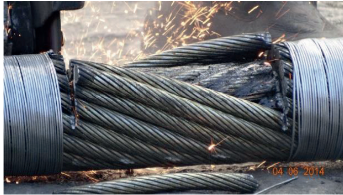
Figure 3 — Alternative serving and cutting method for large diameter rotation-resistant rope
