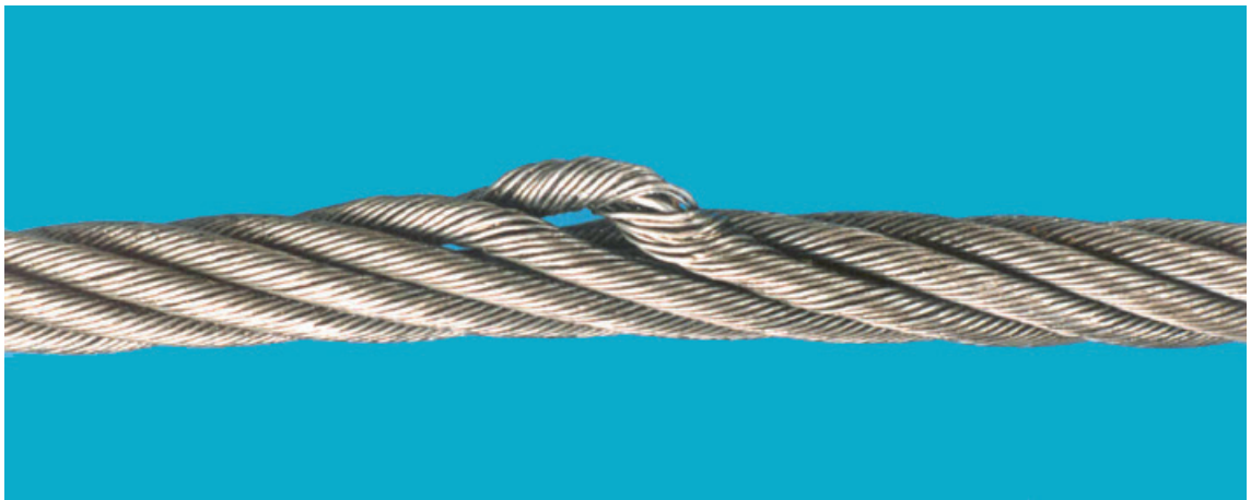
Figure B.13 — Strand protrusion/ distortion
