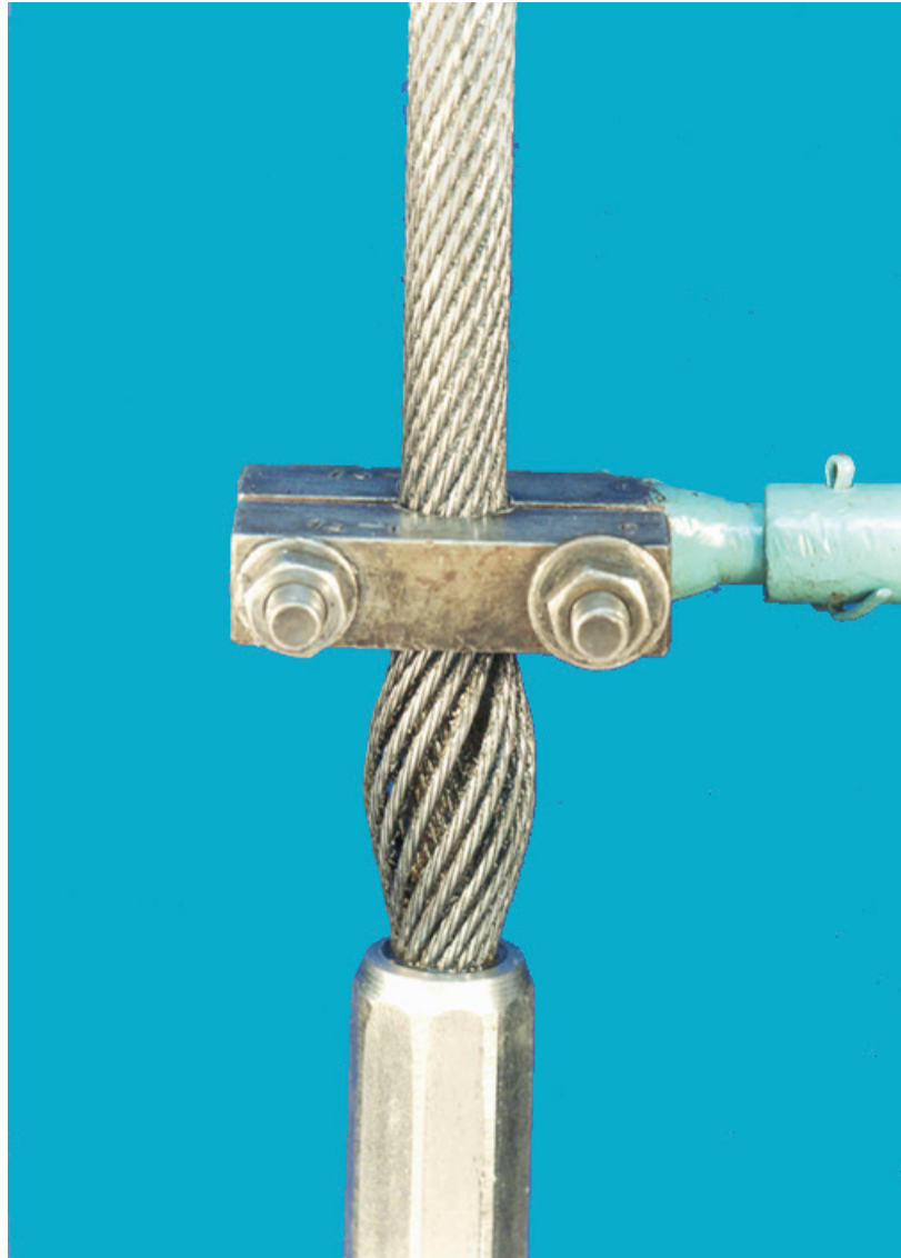
b) At the end of a rope, close to the terminal fitting (zero tension)
