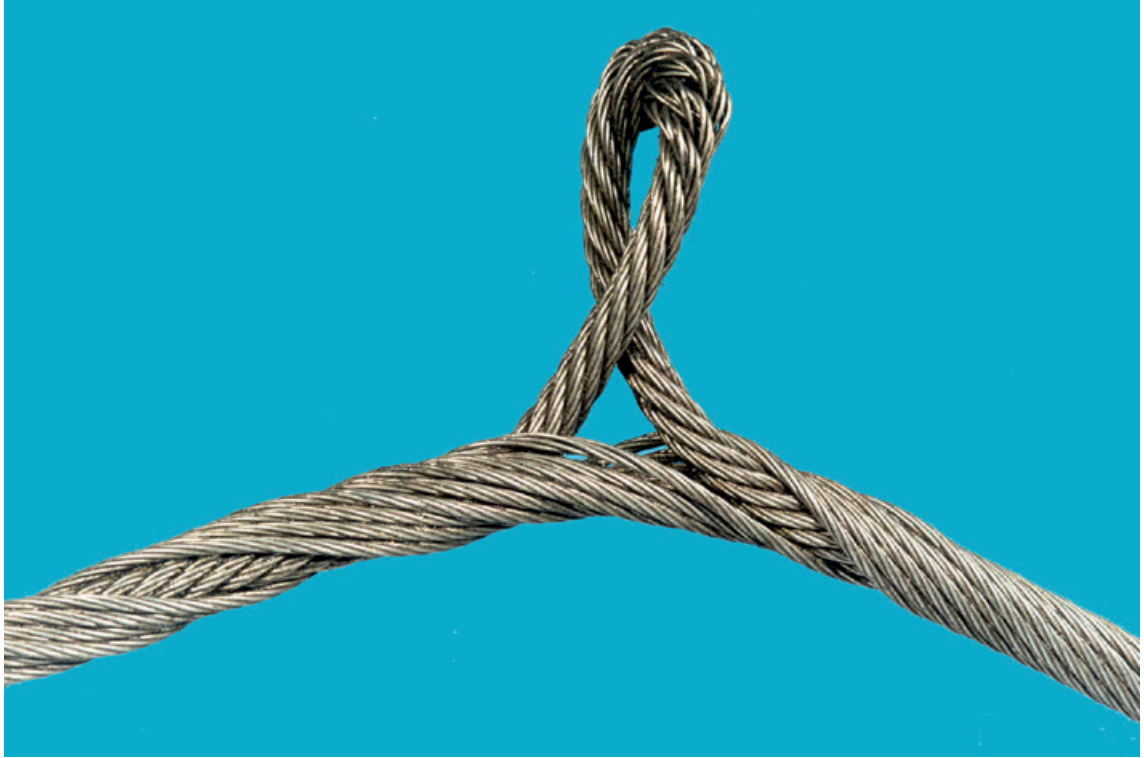
Figure B.12 — Protrusion of inner rope of rotation-resistant rope
