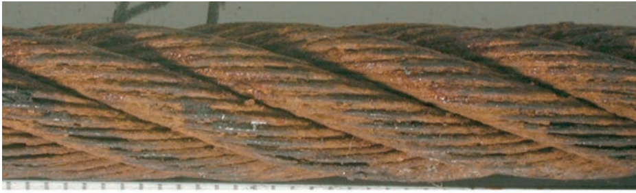
Figure I.4 — Surface heavily pitted and wires quite slack, gaps between wires — Discard immediately
